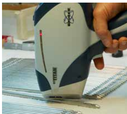
Second Generation S1 TITAN™ handheld XRF analyser from Brucker Elemental.
