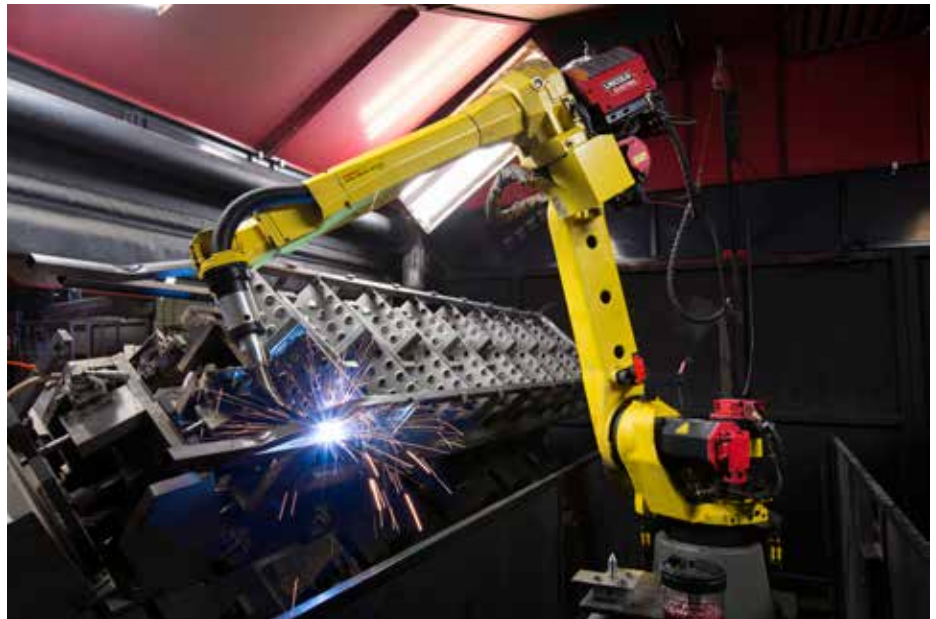
Robotic welding (photo courtesy Lincoln Electric).
