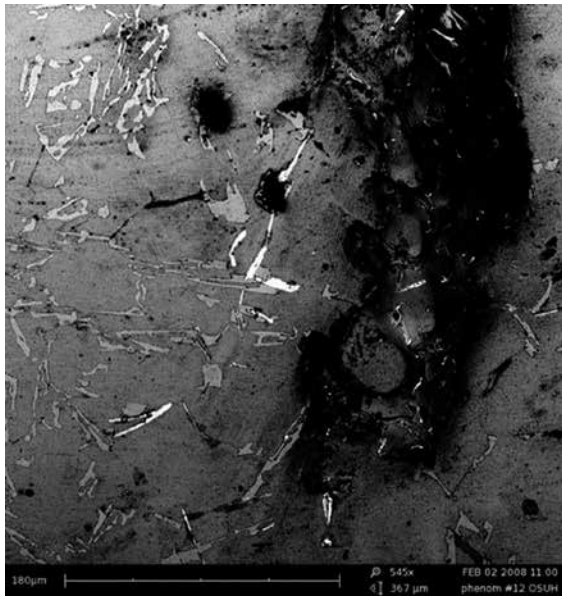
Intermetallics and porosity of an automotive Al alloy (Figure 3).
