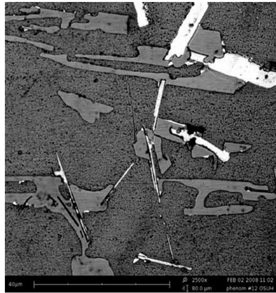
Intermetallics and porosity of an automotive Al alloy (Figure 4).
